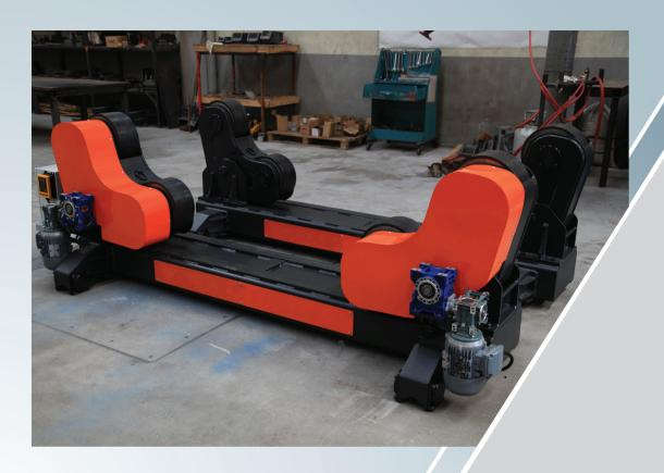
Rotators (Turning Tables) are designed to rotate cylindrical vessels such as tanks, tubes, silos, pipes etc. Rotators are classed depending on the vessel that is being rotated and the vessels weight. Please contact us for technical details and specifications.
